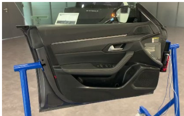
E-Tric Tracks demonstrator: a car door in which the cables have been replaced by the intelligent lining (©SEGULA Technologies)
