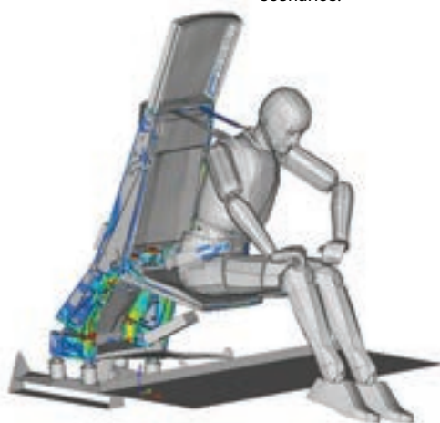
Digital validation of aircraft seat design for crash scenarios.
